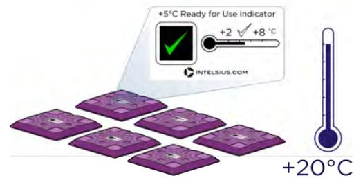
3. The Utektile panels define a fixed payload space where temperature control is maintained. Place one panel in the base of the ORCA insulation, with front label facing upwards then arrange four other panels around the vertical walls of the insulation with the labelled faces inwards. The payload can now be inserted into the space defined by these 5 panels. The remaining panel can now be added to the top with the label facing downwards.
