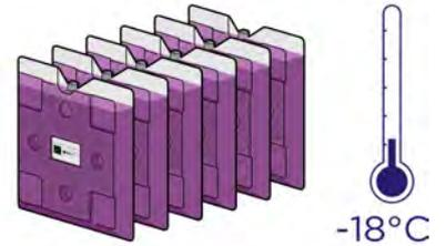
2. Take the frozen Utektile panels from the freezer space and lay them label side up in a room temperature environment ( $+20^{\circ}\text{C} \pm 3^{\circ}\text{C}$ ). Ensure they are well spaced with sufficient airflow over the labelled face. The panels require a minimum time of 40 minutes at this temperature in this space before they are ready for use. These panels can remain in this space for a further 20 minutes, before they will need to be returned to the freezer environment.
